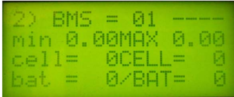
Fig. 4. Menu 2: the minimum and maximum voltages.
