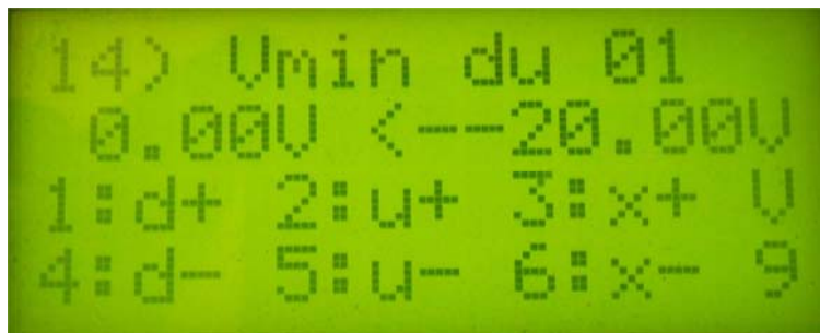
Fig. 16. Menu 14: the minimum voltage per cell.
